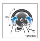
① Turn VOLUME dial to adjust the value of the level, balance or style, then press this dial.
